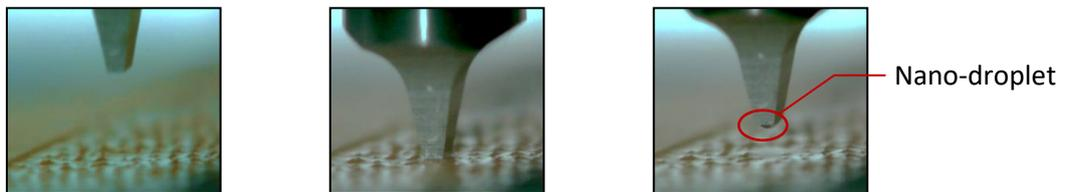
*Fig.: (a-b) A metallic gripping tool coming in contact with an imbibed porous media, creating a liquid bridge. (c) After the rupture of the liquid bridge, the tool leaves with a droplet of a few nanoliters.*
